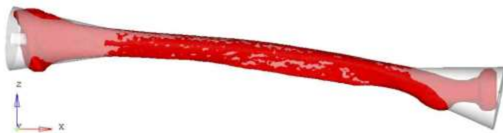
図 4-8-16 A comparison between radius FE model and test piece model
